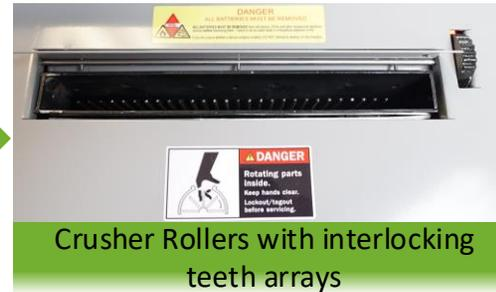
Crusher Rollers with interlocking teeth arrays
